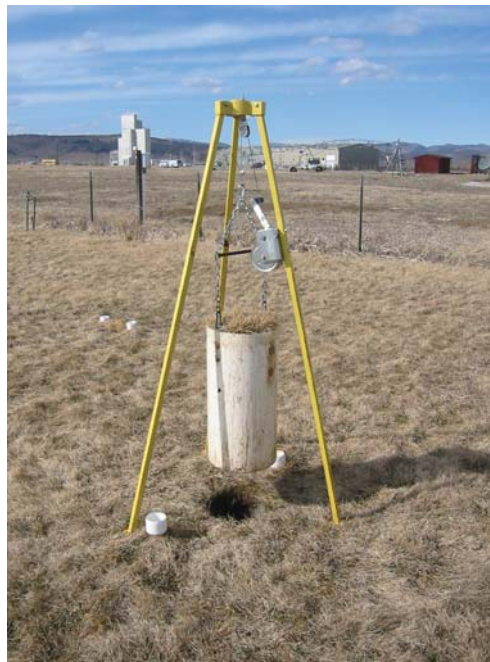
Figure 1. One of twenty-four lysimeters used during the nutrient leaching experiments conducted at the Agricultural Engineering Research Center at Colorado State University.
