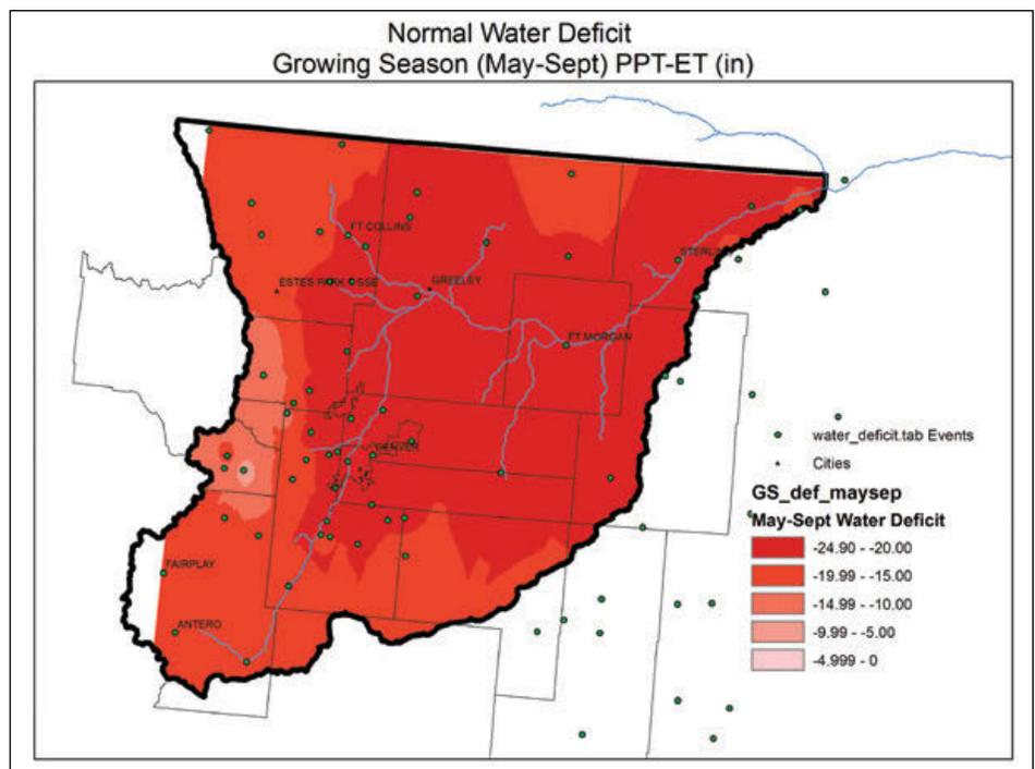
Figure 6. Using climate normal and the Blaney-Criddle evapotranspiration (ET) calculation, the map shows the normal water deficit of the South Platte basin by subtracting ET from precipitation.
