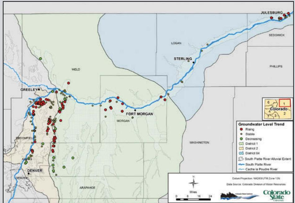
Figure 2. Groundwater Depth Trends Over 2000-2012 for Observation Wells with Complete Records for the Period, where red dots indicate rising water levels over the past decade.
