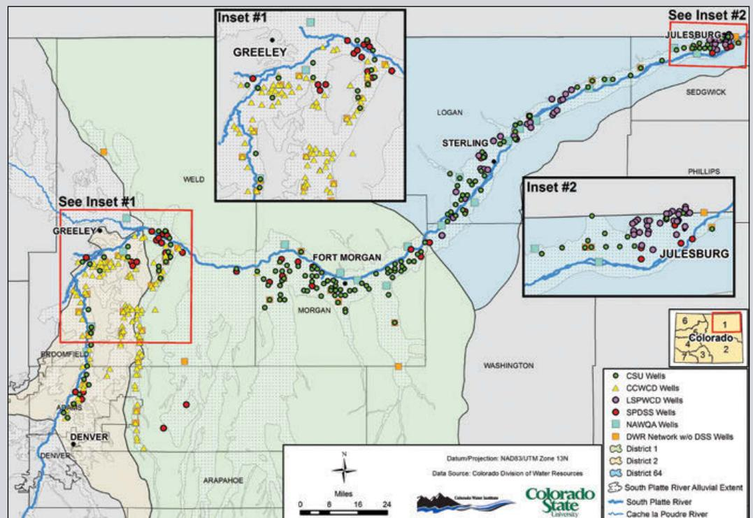
Figure 1. Observation & Monitoring Wells of the South Platte River Alluvial Aquifer
