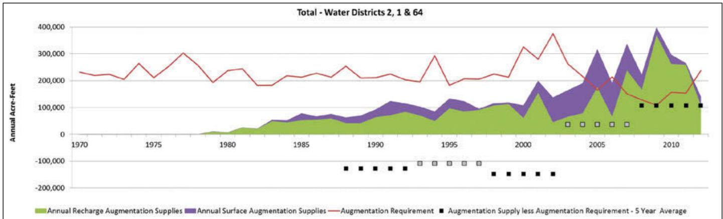
Figure 4. Total annual surface and groundwater augmentation supplies versus estimated potential augmentation requirements, and five-year average augmentation supplies less potential augmentation requirement in water districts 2, 1, and 64.
