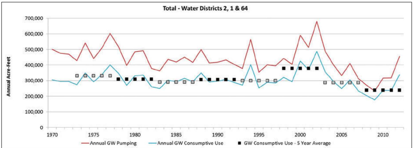
Figure 2. Total Estimated Annual Pumping and Groundwater Consumptive Use in Water Districts 2, 1, and 64. Data Source: CO DWR HydroBase Version 20130710.
