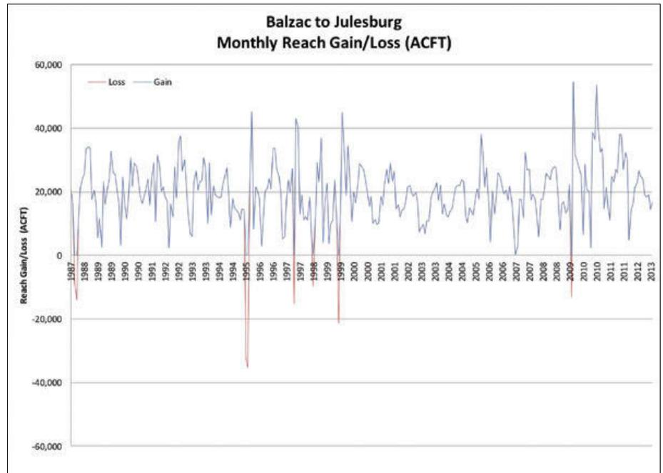
Figure 4. An example gain/loss computation created from TSTool commands.
