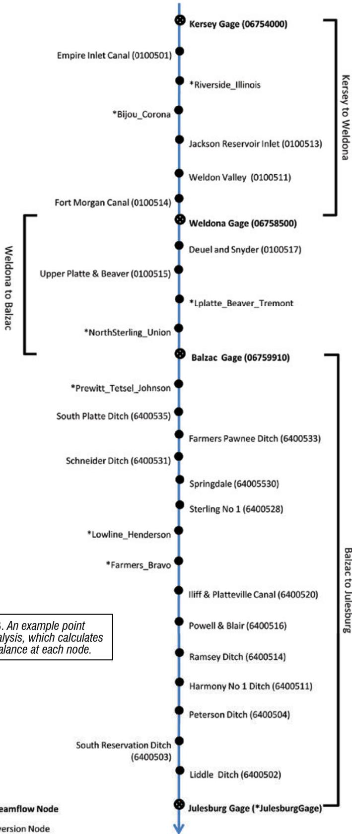
Figure 3. An example point flow analysis, which calculates water balance at each node.
