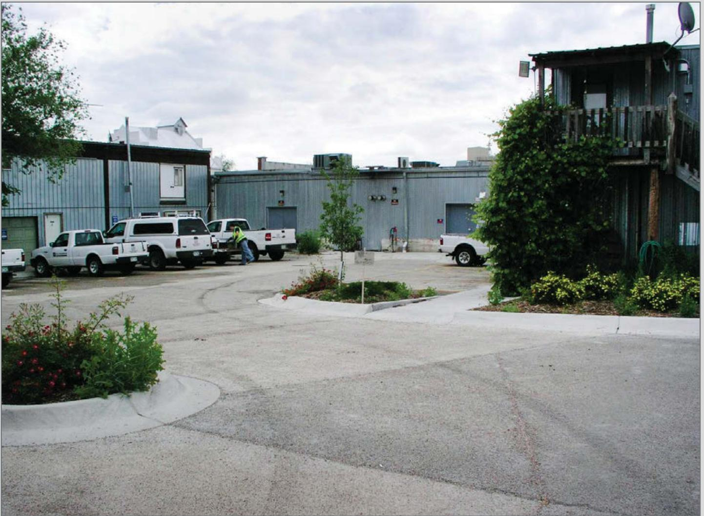
Figure 9. CTL Thompson driveway and parking lot is porous concrete and can infiltrate all the runoff from surrounding roofs and the parking area.
